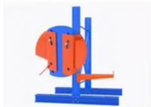
Step 4: Install the cantilever beam
